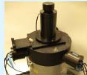
NPL Triple-to-Double Coincidence Ratio (TDCR) detection chamber assembly, with the housings for the three photo-multiplier tubes (PMTs) visible
