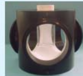
TDCR optical chamber where the Liquid Scintillation vials reside during measurement. The holes accept the 3 PMTs
